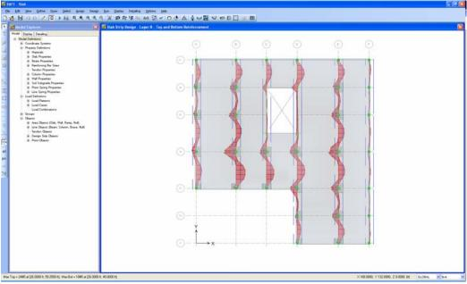
Figure 41 Layer B reinforcing
