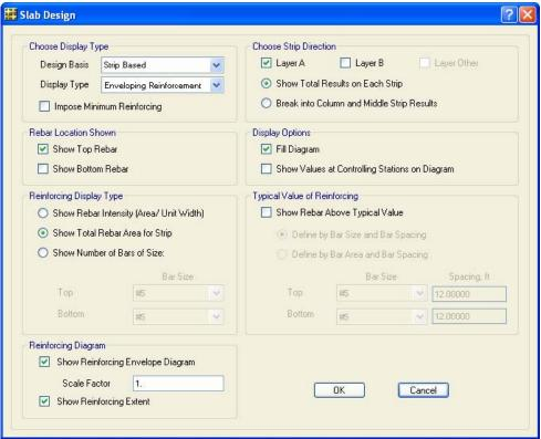
Figure 40 Slab Design form
