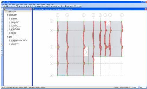
Figure 91 Layer B Long-Term Compressive Stresses
