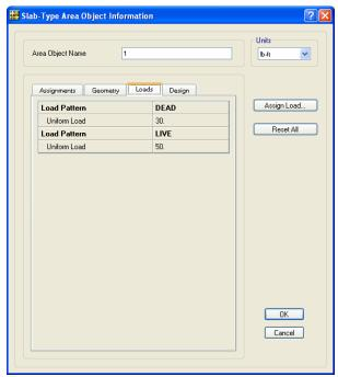
Figure 36 Slab-Type Area Object Information form
