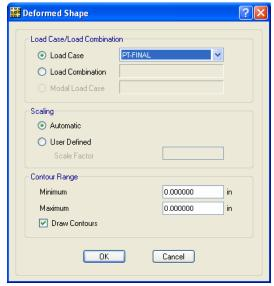
Figure 87 Deformed Shape form
