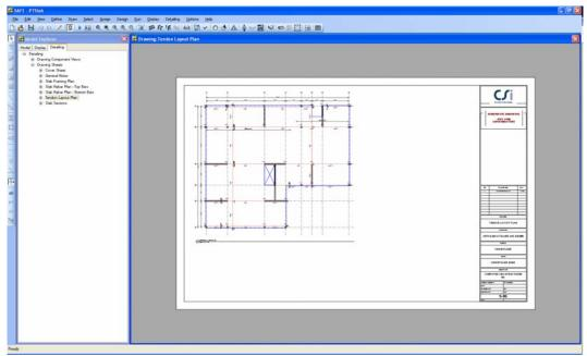
Figure 95 Tendon Layout Plan
