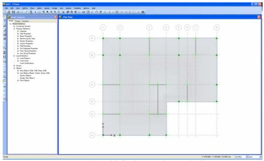
Figure 75 The model after drawing columns and walls
