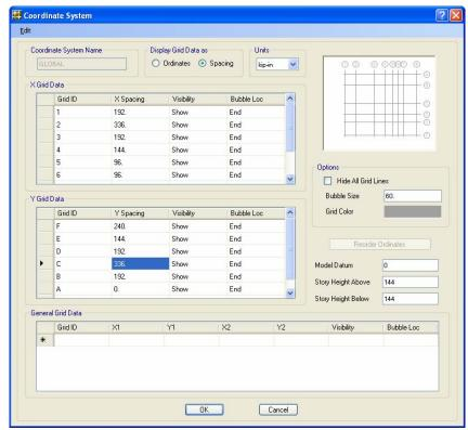
Figure 55 Coordinate System form
