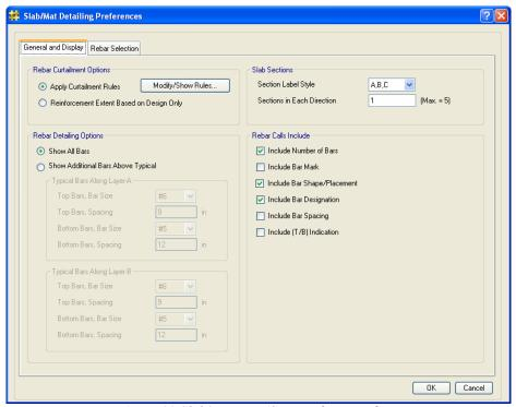
Figure 93 Slab/Mat Detailing Preferences form
